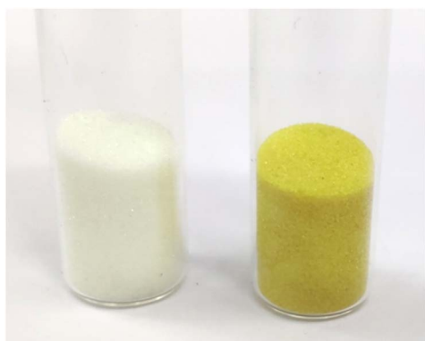
Fig. 16 Colorimetric reaction of DAS (50 \mu\text{M} in MeOH) towards Ni 2+ in solid state.
