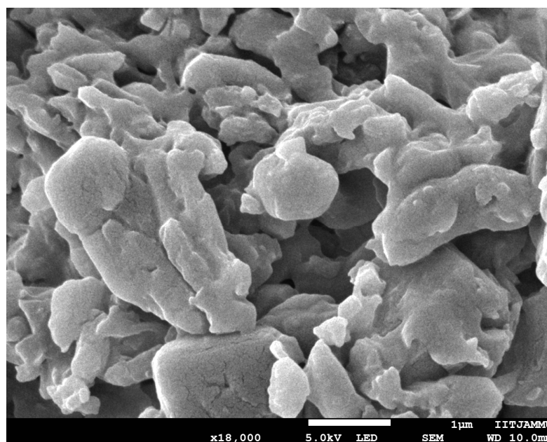
Figure 2. SEM image of coumarin-loaded SLN dispersions.
