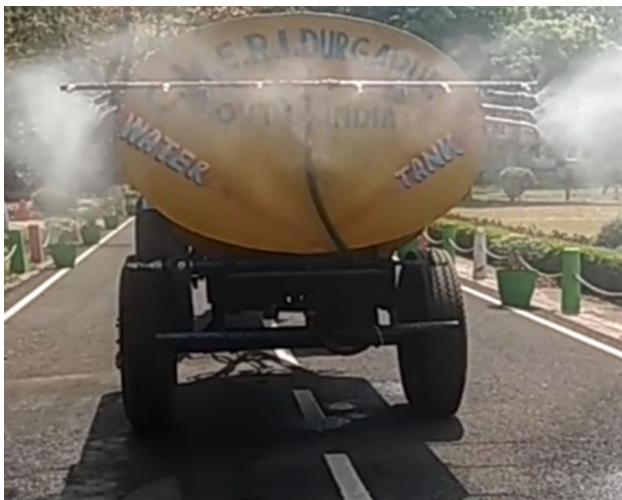
Fig. 2 Road sanitizing unit under operation
