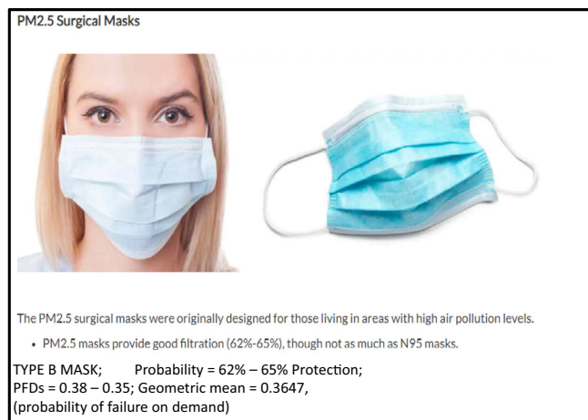
FIGURE 3 PM2.5 surgical mask independent protection layer calculation
