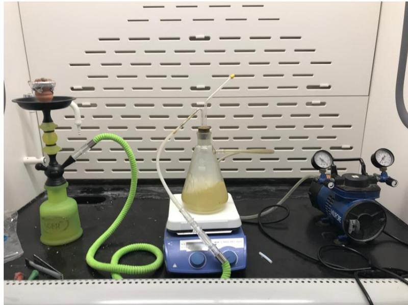
**Figure 1.** A new waterpipe smoking (WPS) setup used to collect smoke residue.
