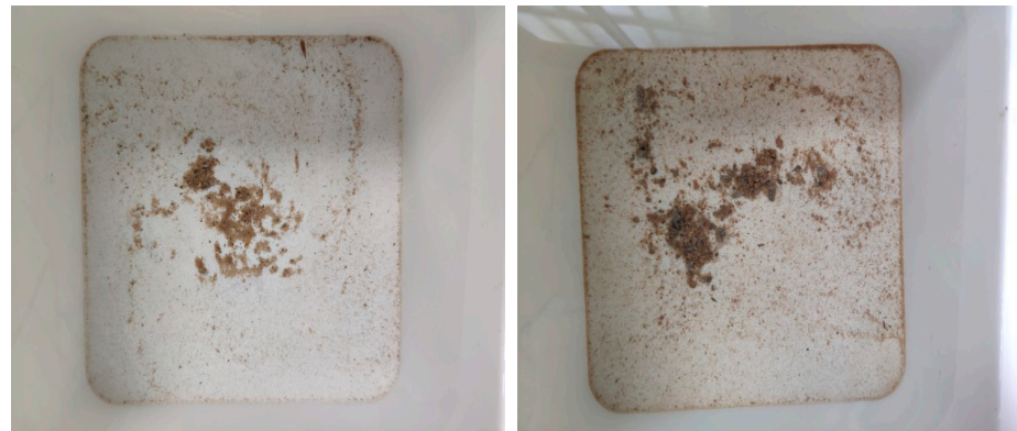
Figure 8. Change in fine gravel content in the corrosive liquid drum.
