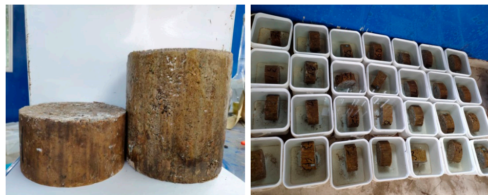
Figure 1. Cement-stabilized macadam samples.
