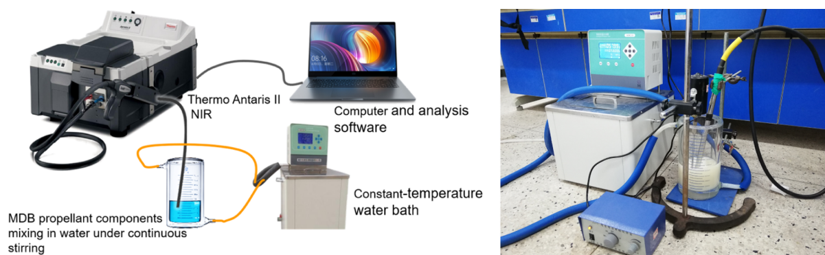
Figure 2. Self-built equipment for evaluation of blend uniformity and terminal point of MDB propellant components: schematic diagram (left) and actual installation picture (right).
