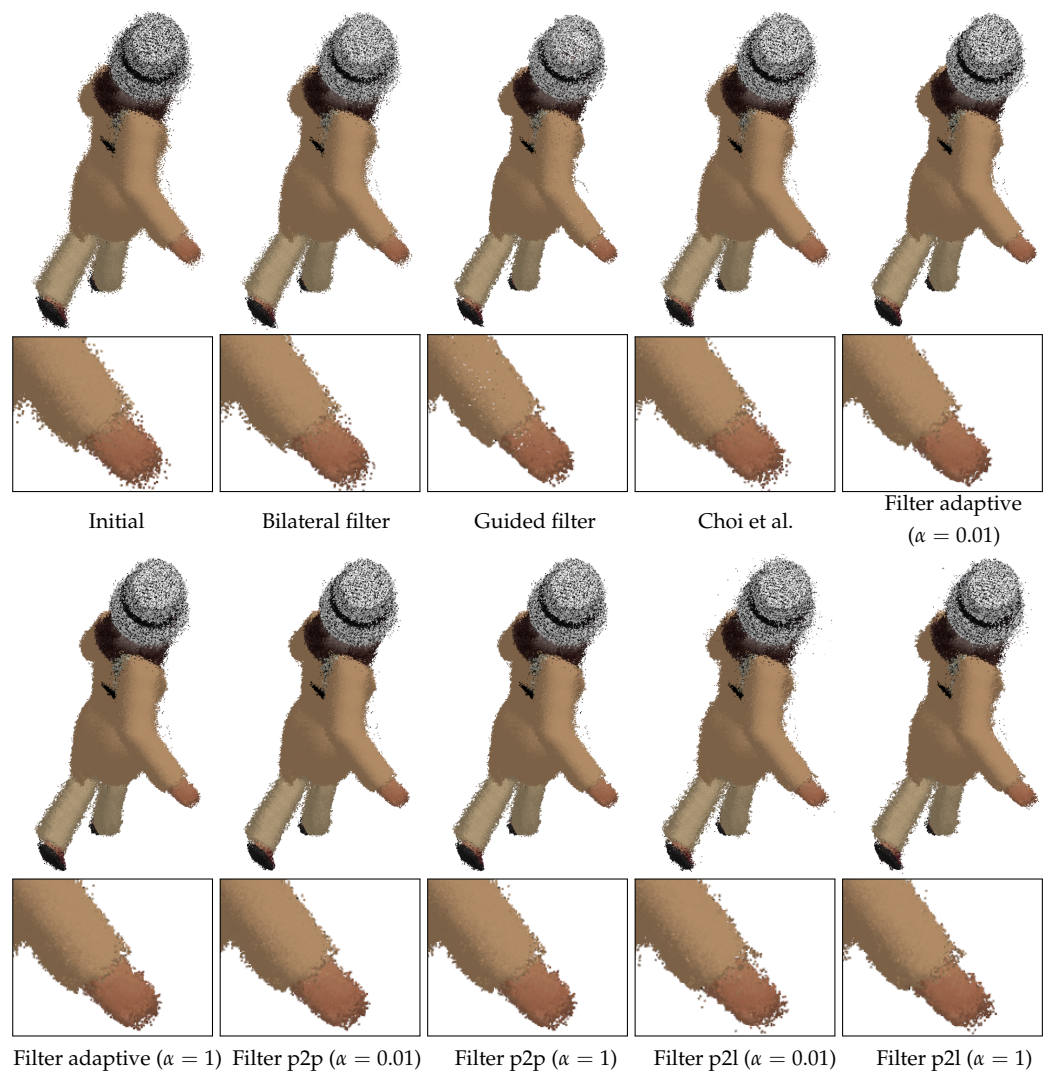
Figure 5. Point cloud rendering results. (First and third rows): Merged point clouds. (Second and fourth rows): Magnified hand regions. We note that neither a preprocessing nor a postprocessing method has been applied to the results.
