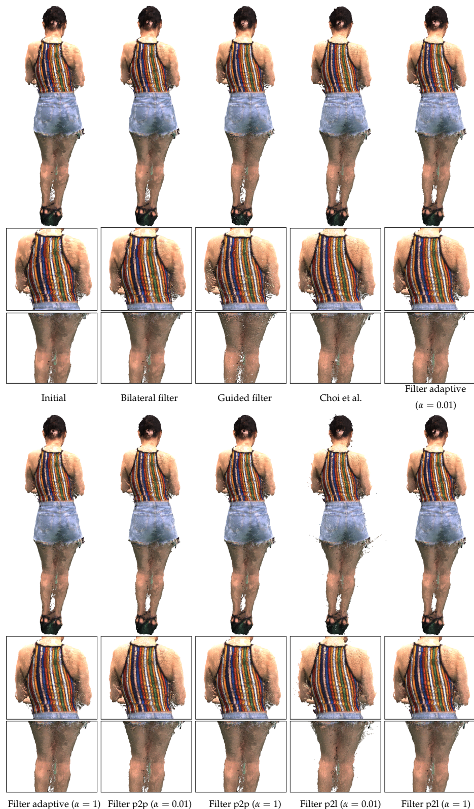
Figure 7. Point cloud rendering results. (First and fourth rows): Merged point clouds. (Second, third, fifth and sixth rows): Magnified regions. We note that neither a preprocessing nor a post-processing method has been applied to the results.
