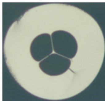
Figure 38. Microscope image of the three holes PCF with suspended Ge-doped silica core. It is combined with fiber Bragg grating and holes are filled with analyte then used as refractive index sensor (Reproduced from [107], with the permission of OSA publishing).
