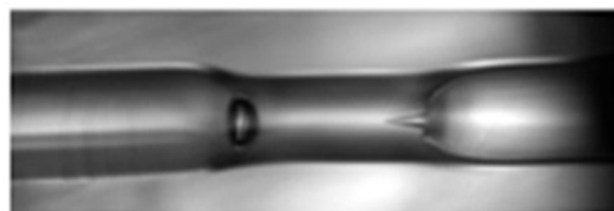
Figure 28. A micro-air cavity is formed by splicing hollow core PCF and SMF for curvature measurement (Reproduced from [90] with the permission of IOP science publishing).
