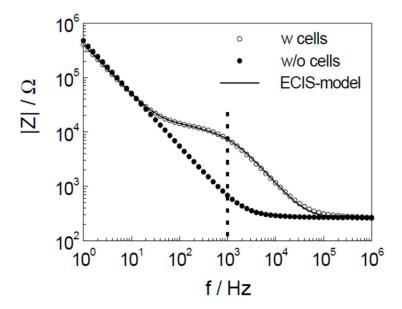
**Figure 5.** CBI spectra with and without cells performed on a gold electrode verifying that frequencies outside of 10 Hz–100 kHz were independent of cell properties. Reprinted from Arndt et al. [45] with permission from Elsevier.
