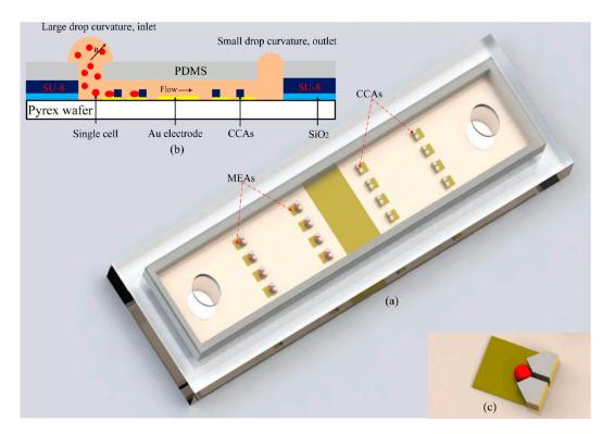
**Figure 11.** (a) 3D image of the sensor chip, which consists of three main parts: microelectrode arrays (MEAs), cell capture arrays (CCAs), and a microfluidic channel with an inlet and an outlet. (b) Cross-sectional view of the MFC with a mechanism of passive pumping. (c) A V-shaped structure for single cell trapping. Reprinted from Nguyen et al. [54] with permission from American Chemical Society.
