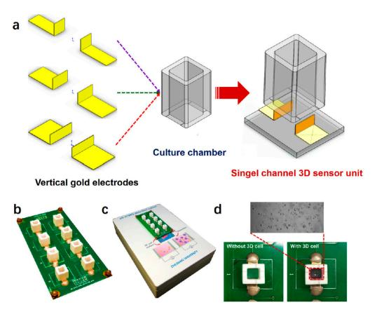
**Figure 7.** Schematic of the different parts of 3D electric cell/matrigel-substrate impedance sensing (3D-ECMIS): (a) vertical gold electrodes in a single channel, (b) arrangement of 8 channels on the scaffold, (c) picture of the eight channels in the detection system, and (d) images of the 3D cell-based biosensor before and after seeding the living cells. Reprinted from Pan et al. [76] with permission from Elsevier.
