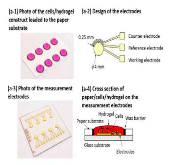
**Figure 9.** Schematic procedure of fabrication of the paper-based CBI sensor. Reprinted from Li et al. [77] with permission from Elsevier.
