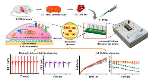
**Figure 13.** Schematic diagram of the drug-induced cardiac side-effect assessment platform with the CBI system and long-term electrophysiology recording platform. Reprinted from Gu et al. [96] with permission from Royal Society of Chemistry.
