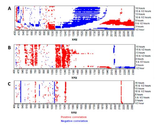
**Figure 14.** Toxin map of endothelial cells (ECV304) response to (**A**) dimethyl sulphoxide, (**B**) saponin, and (**C**) cadmium chloride treatment during 24 h at the frequency range 400–2400 kHz. Reprinted from Gasser et al. [99] with permission from Elsevier.
