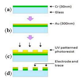
**Figure 1.** A typical fabrication procedure of the sensing substrate used in cell-based impedance (CBI) set up. (a) the glass surface is coated by 30 nm layer of Cr; (b) followed by a 300-nm layer of Au; (c) and (d) Au/Cr layer is subsequently photoetched into interdigitated electrodes. Adapted from Wang et al. [43] under a Creative Commons Attribution License.
