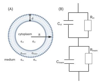
**Figure 6.** (**A**) A diagram of the electric model of the cell according to Maxwell's theory of mixtures. (**B**) Equivalent circuit of the single cell model [26,48].
