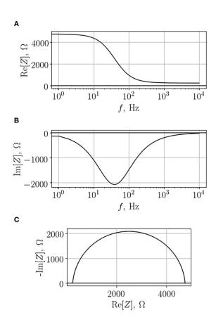
**Figure 4.** Typical electrochemical impedance spectroscopy (EIS) spectra obtained from a monolayer of cells. (**A**) The real component of the Bode plot, (**B**) the imaginary component of the Bode plot, and (**C**) the Nyquist plot in which the real impedance is plotted against the imaginary one. Adapted from Gerasimenko et al. [36] under Creative Commons Attribution License.
