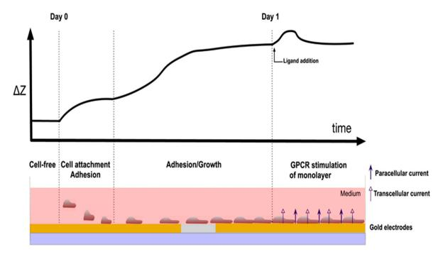
**Figure 2.** Illustration for the CBI-based assay for the detection of cell adhesion and growth. Once a monolayer of cells was formed, subsequent toxicology and drug screening experiments could be performed. Adapted from Doijen et al. with permission from Elsevier [30].
