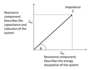
**Figure 3.** Phasor diagram relating the Cartesian and polar coordinates of impedance in the complex plane.
