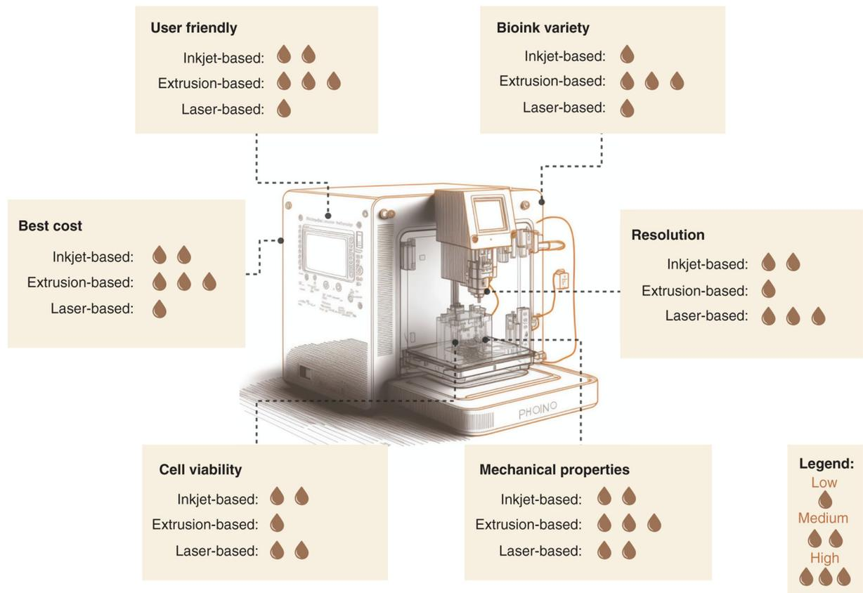
**Figure 2. Comparison of inkjet-, extrusion- and laser-based biprinters for cardiac model development.**
