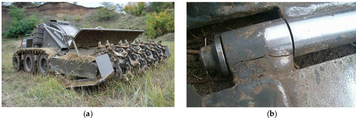
Figure 3. (a) Demining equipment Božena 5 and (b) an image of the weld damage of the currently used steel track caused by its operation.
