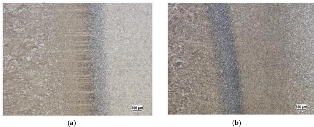
Figure 5. (a) A transfer of the metal being welded (its microstructure) to the area affected by the heat of the material Strenx 960 using the electron beam technology and (b) a transfer of the metal being welded into the area affected by the heat using the laser beam technology.
