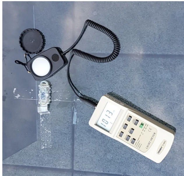
Figure 16. Light measurement calibration of AquaBit.
