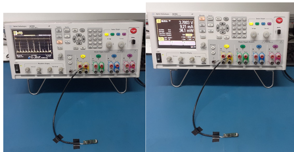
Figure 17. Power consumption measurement of battery lifetime using a DC power analyser.
