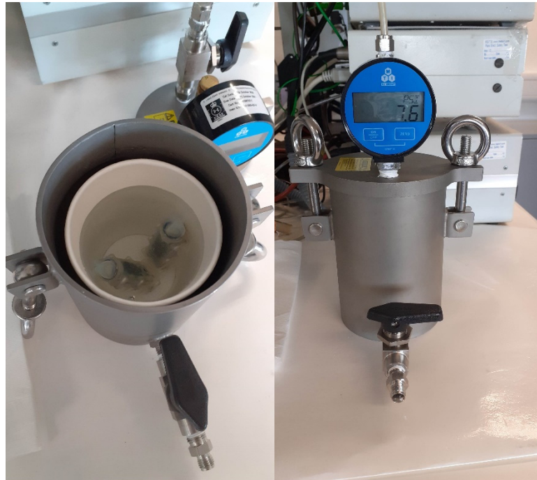
Figure 15. Test setup for the pressure sensor test in water.
