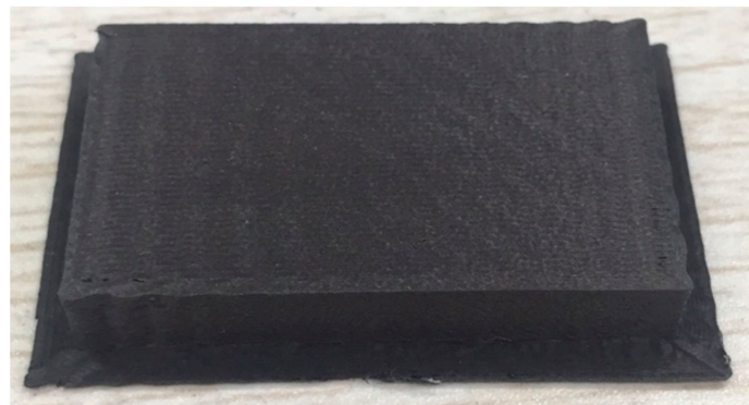
Figure 4. Composite specimen processed by fused deposition modeling (FDM).
