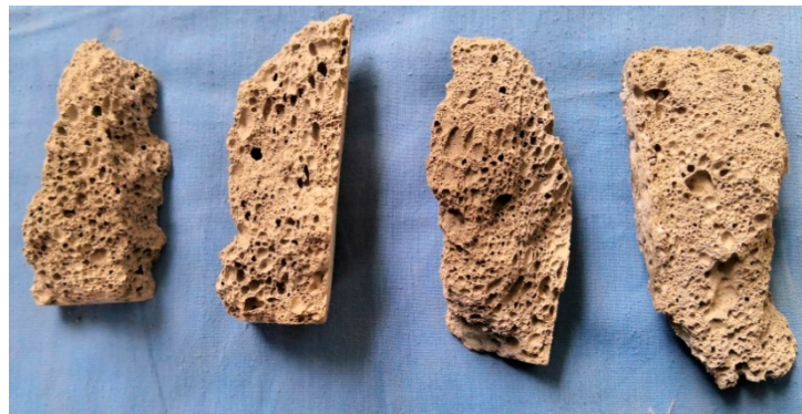
Figure 3. Compression failure characteristics of fly-ash-based foamed geopolymer.
