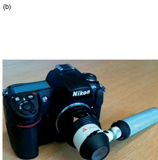
Figure 1. (a) The hand-held OCT probe from the VivoSight 1500 OCT system fitted for this study with a miniature webcam (arrowed), and (b) the Heine Delta 20 dermoscopic attachment to the Nikon DS300 digital camera.
