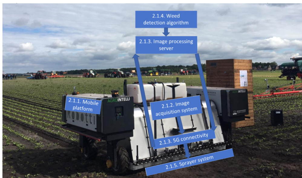
Figure 1. Overview of the robotic precision spraying system. The blocks in the figure highlight the individual components of the robot and show the section number in which the component is described in detail.
