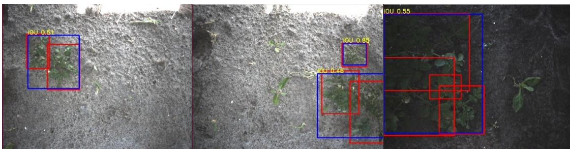
Figure 11. Three examples of multiple potato plants detected as a single potato plant. The red rectangles represent the ground-truth annotations and the blue rectangles represent the detections. The detection resulted in a correct spraying action by the robot, hitting the potato plants. These plants are counted as a TP .
