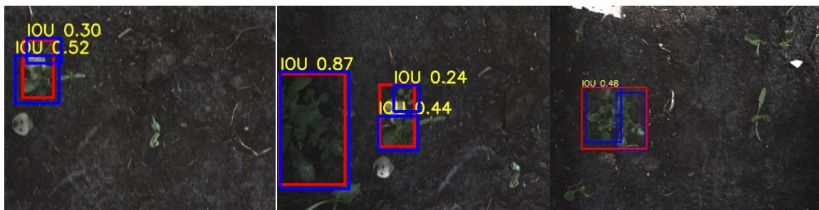
Figure 12. One example of a potato plant detected as two potato plants. The red rectangle represents the ground-truth annotation and the blue rectangles represent the detections. The multiple detections resulted in a correct spraying action. This single potato plant (red rectangle) was therefore counted as one TP .
