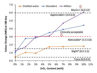
**Figure 2.** Line graph showing the colour change according to NBS unit system in specimens immersed in DW, Steradent (STD) and Milton (MIL) for 180 days.
