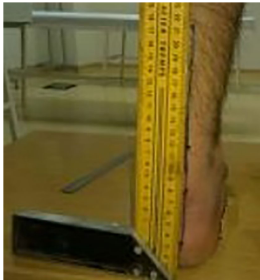
Figure 3. Adjustment of the height of inserted insole into the arch of foot. The height of the insole was adjusted manually until degrees of the line was 90° perpendicular to the ground, which is measured by using a miter.
