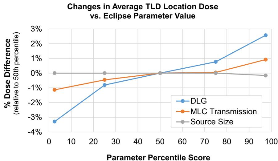
FIG. 2. Average changes in dose calculated to target thermoluminescent dosimeter locations for IROC-H head and neck phantom plans when parameters of interest are manipulated in Eclipse. Percentile score corresponds to community reported values.<sup>15</sup> DLG = dosimetric leaf gap. [Color figure can be viewed at [wileyonlinelibrary.com](http://wileyonlinelibrary.com)]
