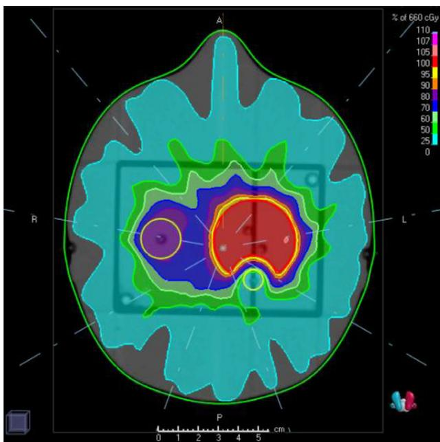
FIG. 1. Axial slice of the nine-field intensity modulated radiation therapy plan developed for the IROC-H H&N phantom. The phantom contains primary and secondary targets planned to be treated at 660 and 540 cGy, respectively. [Color figure can be viewed at wileyonlinelibrary.com]
