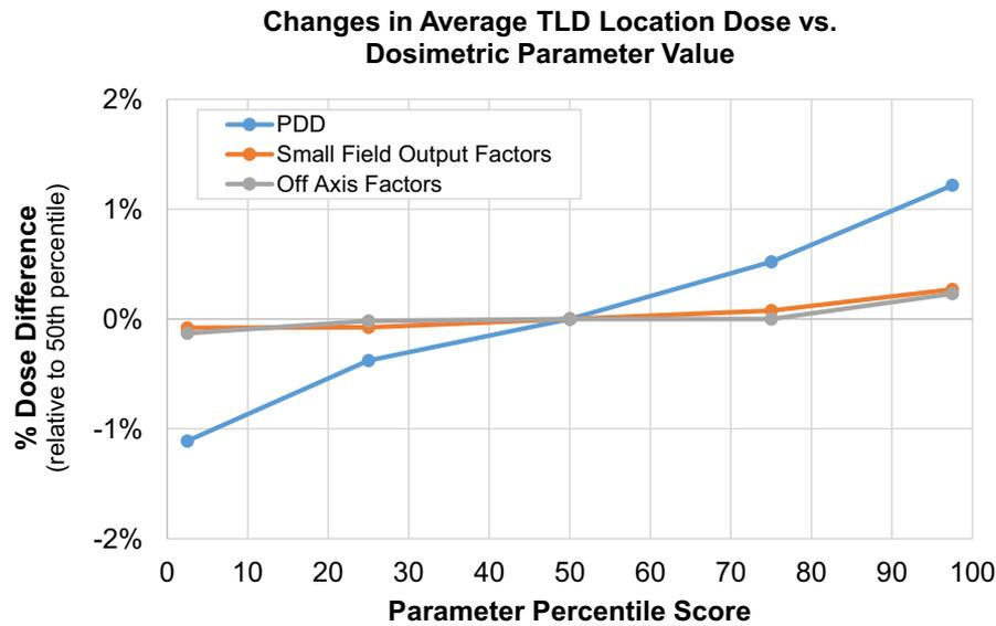
FIG. 8. Average changes in dose calculated to target thermoluminescent dosimeter locations for IROC-H head and neck phantom plans when dosimetric characteristics are manipulated in RayStation according to the documented variations in measurement accuracy from IROC-H site visit data.<sup>14</sup> [Color figure can be viewed at [wileyonlinelibrary.com](http://wileyonlinelibrary.com)]
