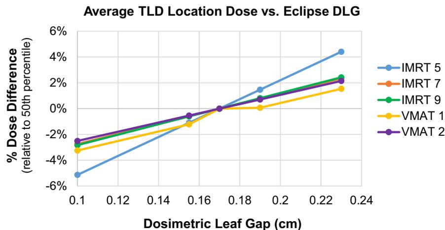
FIG. 3. Changes in average dose for the target thermoluminescent dosimeter locations calculated for each of the five IROC-H head and neck phantom plans following manipulation of the dosimetric leaf gap in Eclipse. Points on the curve correspond to percentile scores from the radiation oncology community for a Varian Base Class machine with a Millennium 120 leaf multileaf collimator. [Color figure can be viewed at [wileyonlinelibrary.com](http://wileyonlinelibrary.com)]
