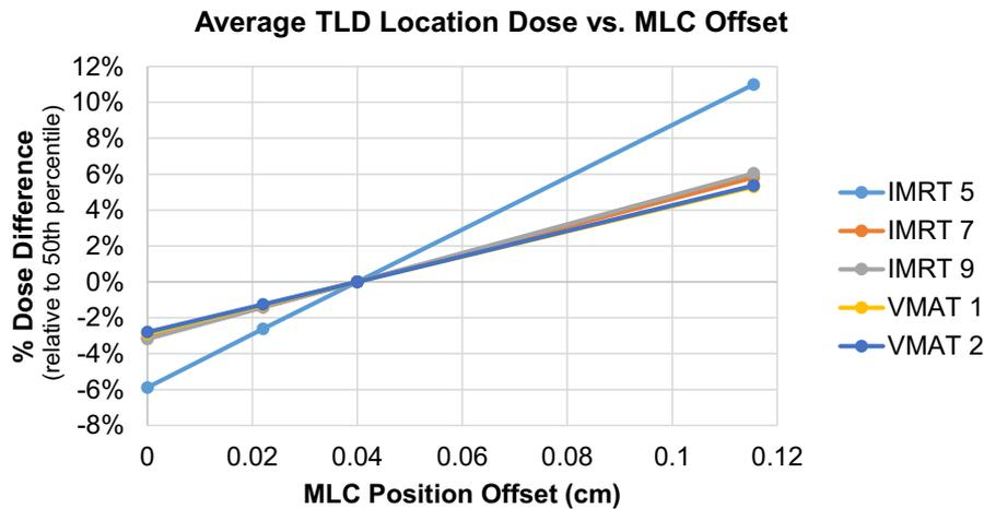
FIG. 6. Changes in average dose for the target thermoluminescent dosimeter locations calculated for each of the five IROC-H head and neck phantom plans following manipulation of the multileaf collimator (MLC) offset in RayStation. Points on the curve correspond to percentile scores from the radiation oncology community for a Varian Base Class machine with a Millennium 120 leaf MLC. [Color figure can be viewed at wileyonlinelibrary.com]
