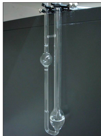
Figure 3: Schematic image of Ostwald viscometer.
