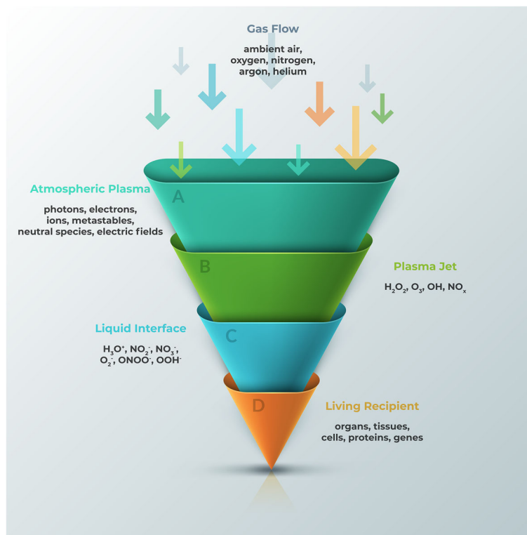
Fig. 2 Hierarchical delivery of plasma-derived reactive species towards stem cells and stem cell niche. (A) Atmospheric plasma phase, and its main components. (B) Plasma jet, and the reactive species contained in its plume. If CAP is used as an indirect approach to activate a stem cell niche, the entire process occurs when plasma jet interacts with the solid interface of a niche. However, if CAP is used to directly stimulate a living recipient, it propagates through a liquid phase first. (C) Liquid interface, and various RONS created upon diffusion through it. (D) The biological effect of plasma penetrates across various levels
