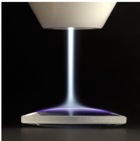
Fig. 3 Interfacial modification of an artificial stem cell niche using CAP. Image was taken when using a handheld plasma device based on piezoelectric direct discharge (PDD) technology. The gaseous plasma jet can be seen exiting the nozzle and spreading over the target surface
