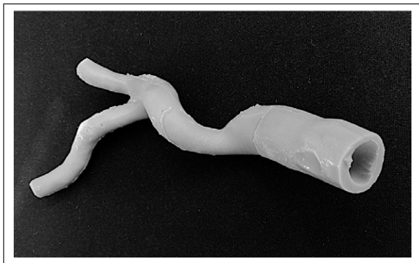
Figure 6. Silicon vessel produced from CT data. At the aortic bifurcation, only the right common iliac artery is visible, giving rise to the external iliac artery (lower left corner) and the internal iliac artery (upper left corner). This model is made from two-component dental cast silicon and is not 3D-printed.
