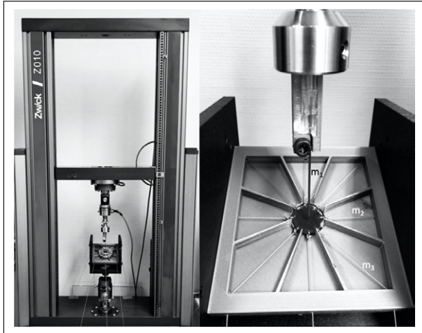
Figure 1. (Left) Zwick electrical testing machine with sample clamp. (Right) Blue silicone Shore A 10 sample with eight Mersilene 1-0 threads tied 45° apart each. The weights with the masses m_1 pull up and down, the weights with the masses m_2 pull left and right. The weights with the masses m_3 pull in diagonal directions.
