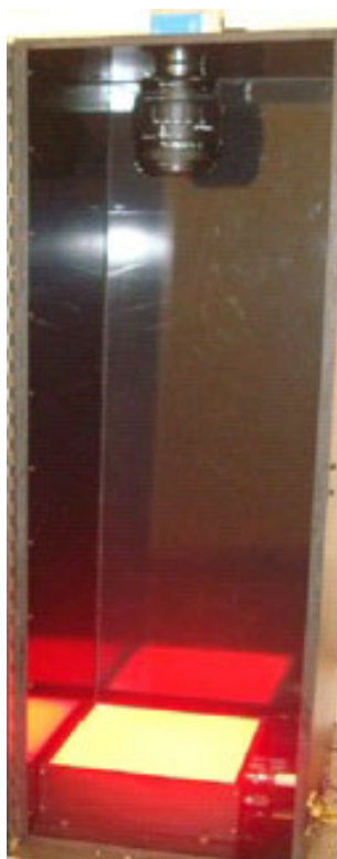
FIG. 1. In-house 2D optical imaging apparatus. The lens is 61 cm away from the LED array, and the light box is 15 × 15 cm 2 . Excess area on the light surface was masked using black construction paper to improve the dynamic range of the system.
