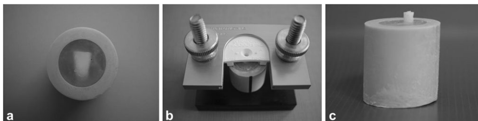
Figure 1 (a) The labial surface of one sample, (b) application apparatus of orthodontic composite on the enamel surface, and (c) the orthodontic composite block over enamel.
