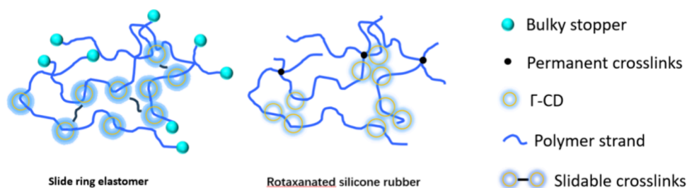
Figure 1. Structural illustration of slide ring elastomer with mobile cross-links and negligible filler–filler interactions and rotaxanated silicone rubbers with permanent cross-links and strong filler–filler interactions.
