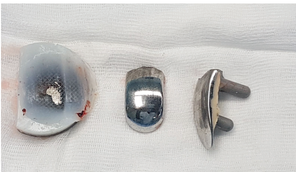
Figure 5. Tibial and broken femoral component of the prosthesis
