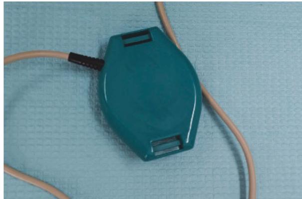
FIGURE 3: Magnetic-light applicator of the Viofor JPS system for local ELF-MF therapy (author's photo).
