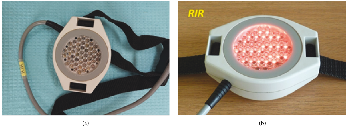
FIGURE 6: Magnetic-light applicator of the Viofor JPS system for local ELF-MF + LED therapy using combined red and infrared light (source: author).
