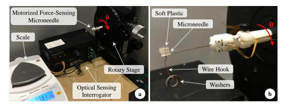
**Figure 4.** (a) Setup for calibration experiments: The force-sensing micro-needle was held horizontal and mounted on a rotary stage to modulate its axial orientation ( $\theta$ ); (b) The microneedle tip was inserted into a soft plastic piece carrying a wire hook. Forces were applied at the needle tip by hanging washers of known weight on the hook.
