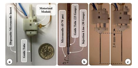
**Figure 2.** (a) Components of the design: force sensitive motorized unit, and the disposable prebent needle (b) Assembled prototype (c) Tool actuation: the microneedle is exposed by retracting the guide tube as much as 2.4 mm.
