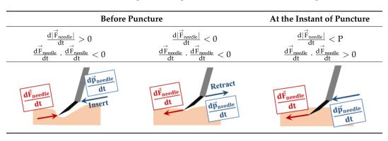
Table 1. Variation of tool tip force and position before and at the instant of puncture.
