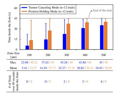
Figure 12. The total time that the needle tip was maintained inside various sizes of zones around the puncture point using the TCM (in blue) versus the PHM (in orange) features. The solid bars show the mean, and the error bars represent the maximum values. The active position holding helps in maintaining the needle tip inside the vein for a significantly longer time, especially for veins smaller than 300 µm [62].
