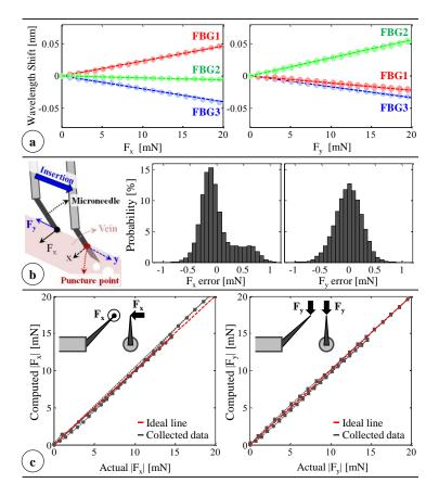
**Figure 5.** (a) Calibration results: linear response for all FBGs when the needle is loaded along x and y axes; (b) The force-sensing coordinates relative to the target vein and the histogram of residual errors in each direction; (c) Computed forces vs. the actual forces along the x and y axes [62].
