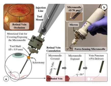
**Figure 1.** (a) Conceptual design of our motorized force-sensing microneedle for retinal vein cannulation; (b) The tool has a thin tip ( $\emptyset$  70 µm) and a modular design that allows for easy integration with robotic devices, such as the Micron handheld micromanipulator.
