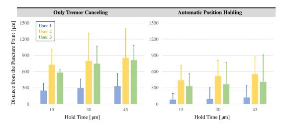
**Figure 14.** Deviation from the puncture point vs. the hold time for each user. The solid bars show the mean distance from the puncture point, and the error bars represent the maximum values. A longer hold time causes the needle to move away from the puncture point more. The automatic position holding mode significantly helps in keeping the needle tip proximal to the puncture point.
