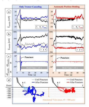
in Figure 11b. In TCM, all components of the position vector fluctuate, especially the z-component due to operator's poor depth perception with the provided 2D microscope view.
