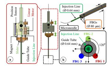
**Figure 3.** Motorized actuation of the tool for retracting the guide tube back and exposing the prebent microneedle. The inner tube of the tool shaft delivers the injection fluid, while 3 FBG sensors on the outer tube sense transverse forces on the microneedle. (**a**) The inner tube of the tool shaft delivers the injection fluid, while (**b**) 3 FBG sensors on the outer tube sense transverse forces on the microneedle.
