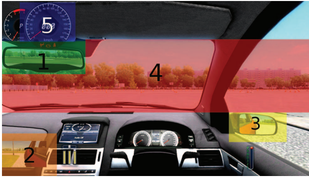
Figure 5. Illustration of each area of interest. (1) Rear-view mirror ( 16^\circ \times 5^\circ ), (2) passenger-side mirror ( 12^\circ \times 5^\circ ), (3) driver-side mirror ( 19^\circ \times 7^\circ ), (4) roadway ( 58^\circ \times 27^\circ at maximum length and height), (5) speedometer ( 12^\circ \times 9^\circ ). See the online article for the color version of this figure.
