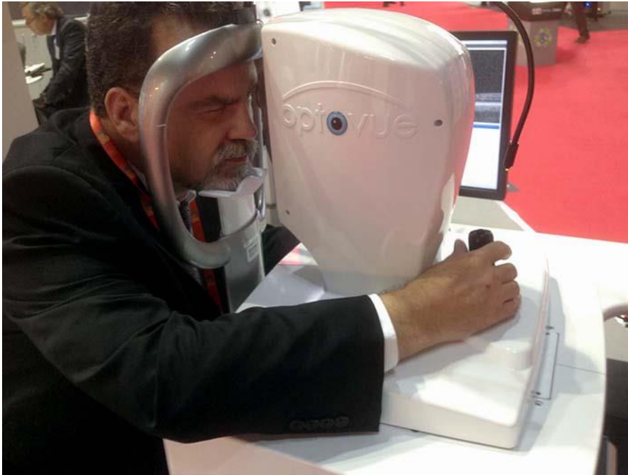
Fig. 2. Operator position during self-OCT angiography (Optovue Avanti RTVue XR). While looking at the fixation target, the instrument body is moved with the control lever using the right hand.
