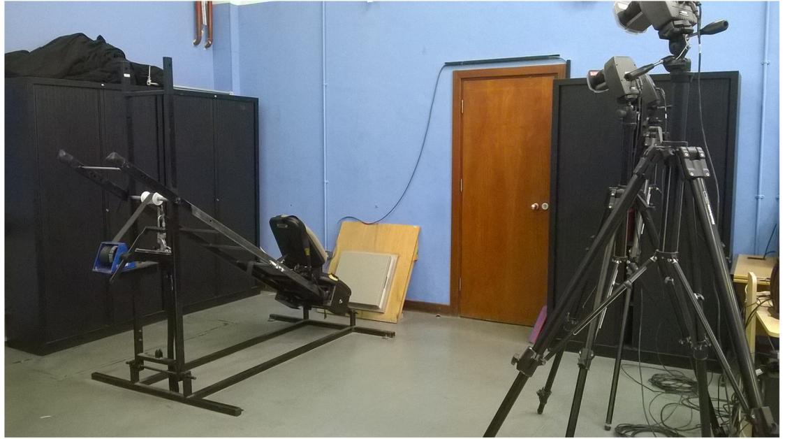
**Fig 1.** Image showing the experimental set-up for hopping trials within the sled-based system.
