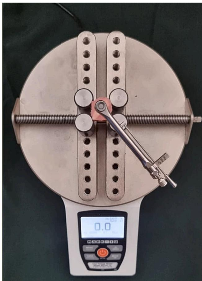
**Fig. 2.** Reverse torque analysis of the titanium implants (Mark-10 Corporation, 11 Dixon Avenue, Copiague, NY 11726 USA).
