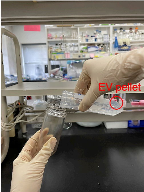
Figure 4. Decantation of the supernatant to a polycarbonate ultracentrifuge bottle with the part of the tube with EV pellet (red circle) facing upward
