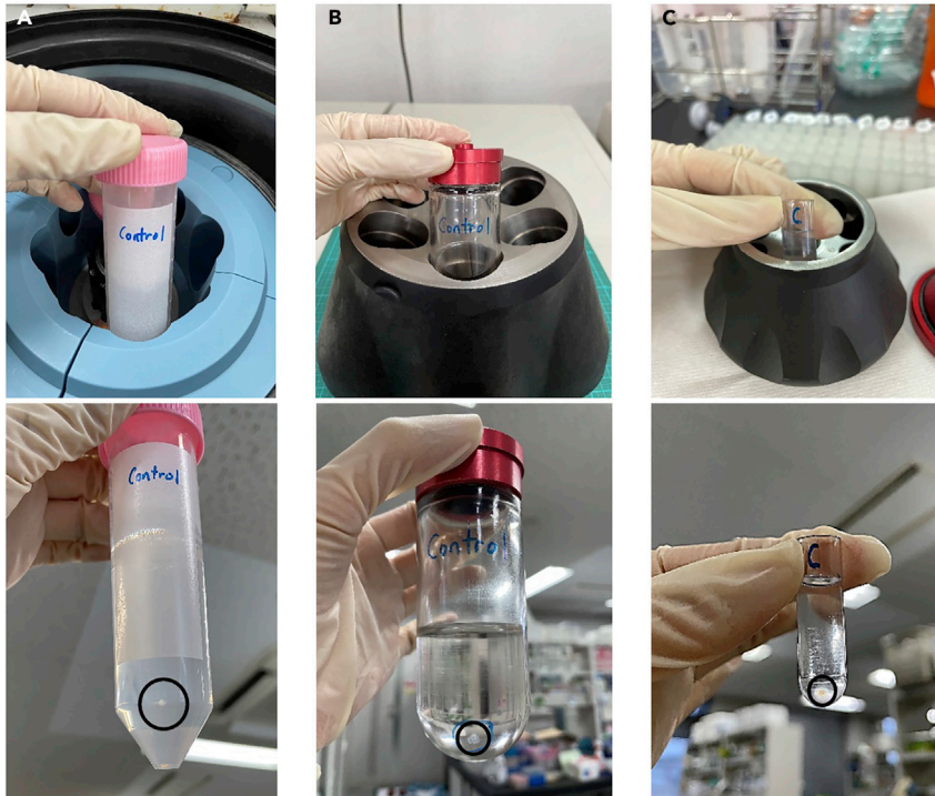
Figure 3. Setting of the centrifuge tubes in rotors and the appearance of the pellet after the centrifugation for each preparation
