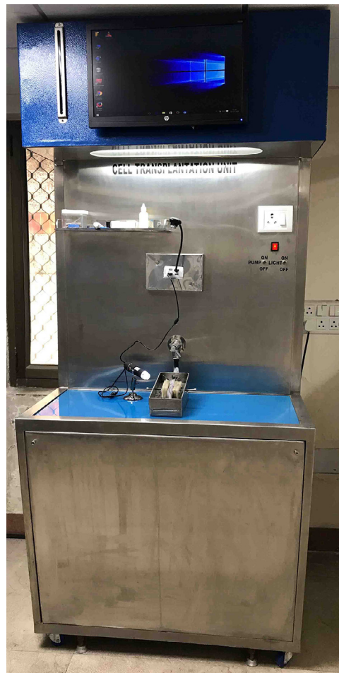
Fig. 1. View of surgery table. The surgery table has an inlet and outlet for water flow. Water containing the anaesthetic agent from the lower tank was raised to the upper tank by using a water pump; the water descended under gravity, passed through the operculum of the fish that was placed inside the chamber.
