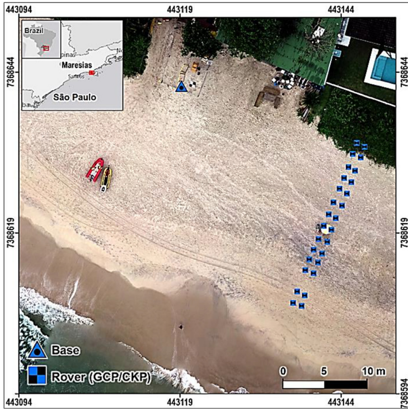
Fig. 3. Location of beach surface generated by SfM-MVS, Base, and Rover GNSS with GCP and CKP locations.
