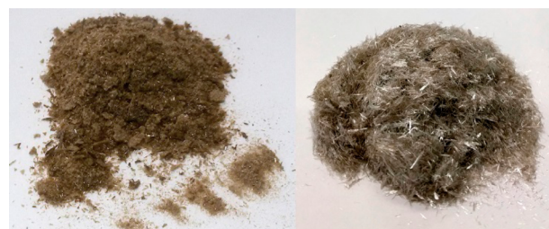
Figure 2. Comparison of the solids obtained after precipitation of di- p -tolyliodonium triflate ( 3a ) produced either in batch (left) or flow (right).
