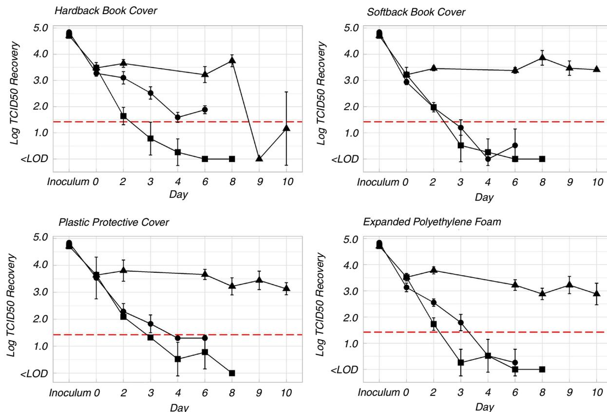
**FIGURE 3** Comparison of storage temperature on the inactivation of SARS-CoV-2  $\pm$  95% confidence interval. (●) indicates Ambient; (▲) indicates Cold; (■) indicates Warm; (---) indicates LOQ
