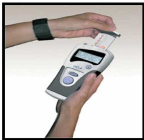
Fig 2: The oral fluid nanosensor test (OFNASET)
