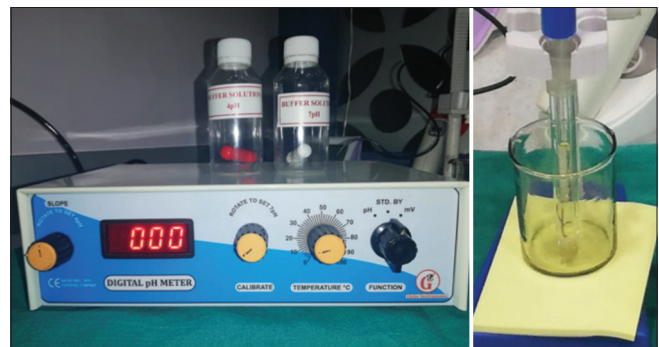
Figure 3: The digital pH meter used for salivary pH analysis and buffering solutions of 4 pH and 7 pH. The tip of pH bulb immersed in the beaker to take the reading
