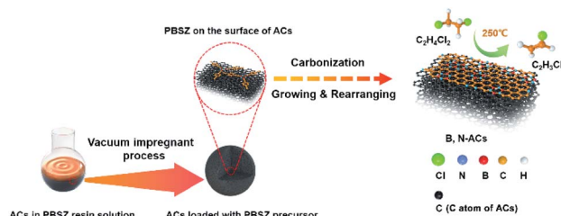
Scheme 2 Schematic representation of the synthesis of B,N-ACs.
