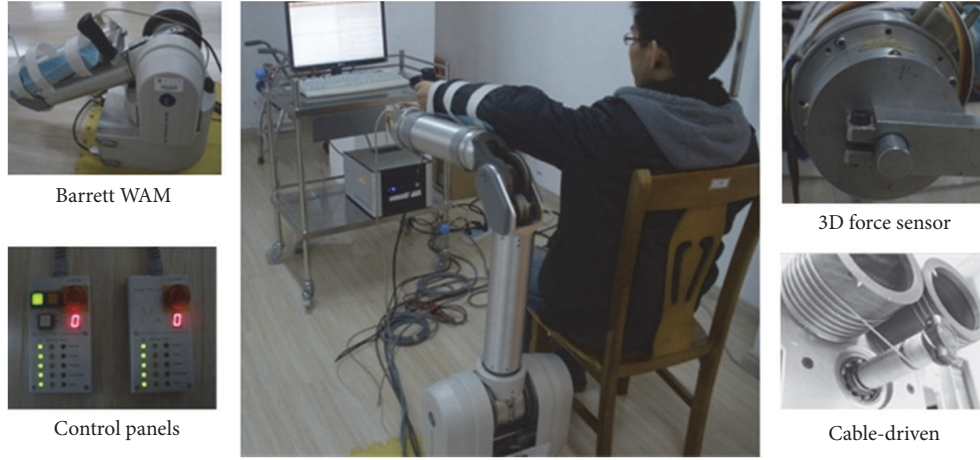
FIGURE 3: Hardware of the WAM upper-limb rehabilitation system.
