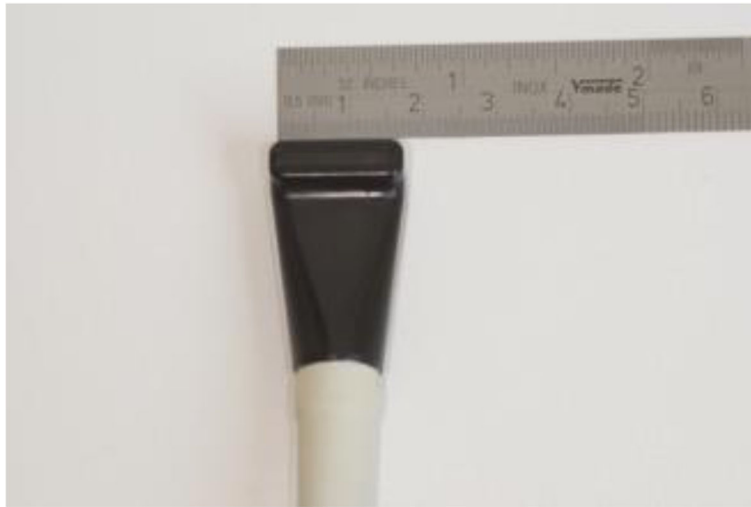
Fig. 2 High-frequency probe (up to 60 \mu m, model L30-8, Mindray Innovation Center, Mindray North America, San Jose, CA, USA) with the size of a toothbrush (30 \times 18 \times 12 mm)
