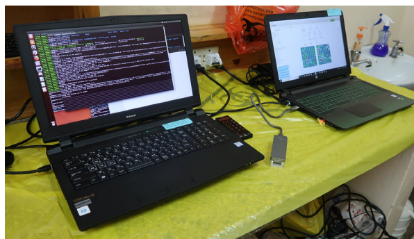
Figure 1. Our portable system for rapid bacterial composition determination. The right PC is connected to the MinION sequencer and handles the sequencing data, while the left PC processes the incoming data simultaneously via a LAN cable. All experiments, including sequencing and analysis, were performed at the University Teaching Hospital in Zambia.
