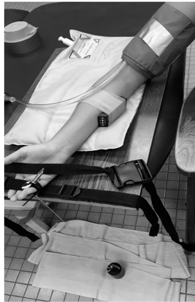
Figure 1. Experimental arrangement. The near-infrared spectroscopy (NIRS) device was placed in the medial (as shown) and lateral positions of the body of the forearm flexor muscles. A blood pressure cuff was placed proximal to the NIRS device. Manual exercise with a 1000 g weight was used to activate finger flexor muscles individually. Subjects were tested in a seated position with a pad under the elbow for support.
