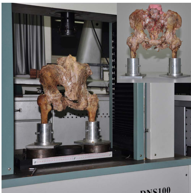
Figure 3. The load cell and jig used to position the pelvis and femur. Test set up: The pelvis is mounted in the up right position, simulating a double-limb stance, free movable in all three planes. The axial load is applied through the forth lumbar vertebra. The fracture dislocations, under axial loading were analysed. Insert at top right = Test set up in anterior-posterior view. doi:10.1371/journal.pone.0082993.g003
