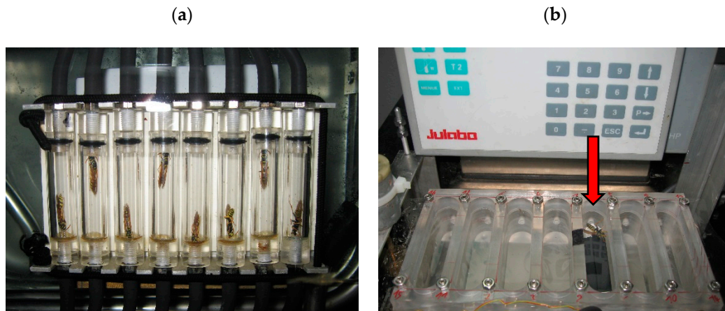
Figure 1. (a) Eight measurement chambers to measure the CO 2 production rate of active and resting wasps ( Polistes biglumis ). (b) Seven measurement chambers in the water bath to measure the endothermic activity and CO 2 production rate of active and resting wasps ( Polistes biglumis ). The arrow indicates the stocked measurement chamber.
