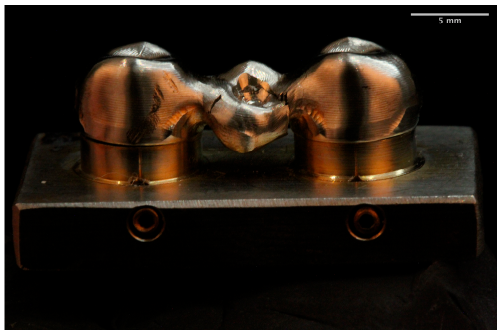
Figure 3. Milled metal framework fracture.
