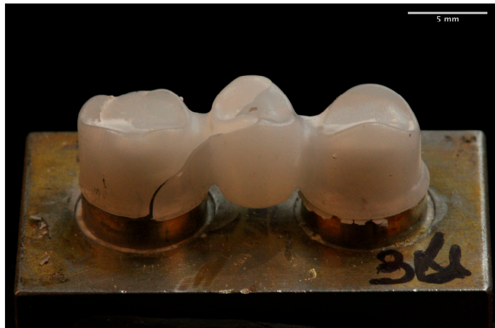
Figure 4. Zirconia framework fracture.
