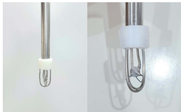
Fig. 1 The recently developed thermocouple sensor based on the work from University of Oxford.
