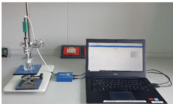
Fig. 3 The testing setup for the proposed device. The measurement was performed by fully submerging the sensing element into the sample.
