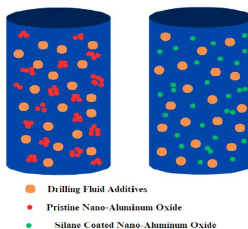
Figure 6. Dispersion of NPs in drilling fluids.
