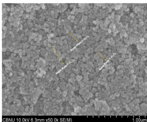
Figure 4. Surface morphology of P- $\text{Al}_2\text{O}_3$  NPs.
