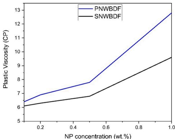
**Figure 8.** Plastic viscosity at different concentrations of P-Al<sub>2</sub>O<sub>3</sub> and S-Al<sub>2</sub>O<sub>3</sub> NPs.
