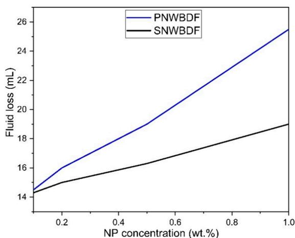
**Figure 13.** Fluid loss at different concentrations of P-Al<sub>2</sub>O<sub>3</sub> and S-Al<sub>2</sub>O<sub>3</sub> NPs.
