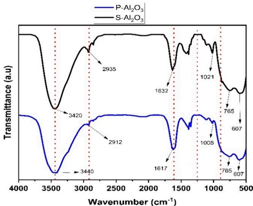
**Figure 2.** FTIR analysis of P-Al<sub>2</sub>O<sub>3</sub> and S-Al<sub>2</sub>O<sub>3</sub> NPs.
