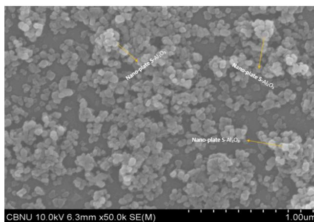
Figure 5. Surface morphology of S- $\text{Al}_2\text{O}_3$  NPs.
