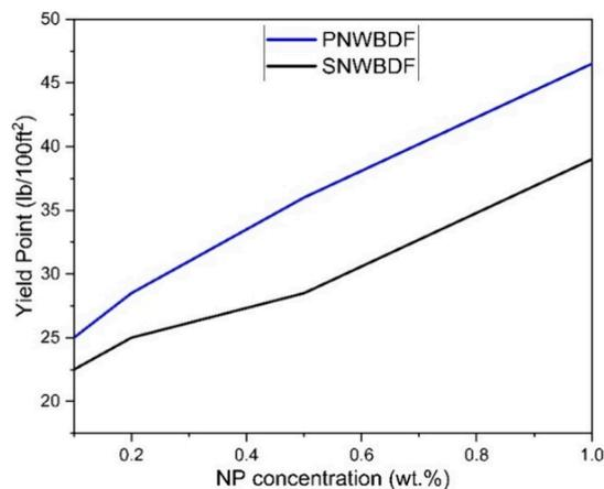
**Figure 10.** Yield point at different concentrations of P-Al<sub>2</sub>O<sub>3</sub> and S-Al<sub>2</sub>O<sub>3</sub> NPs.
