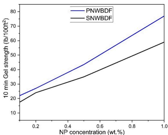
**Figure 12.** 10<sub>min</sub> gel strength at different concentrations of P-Al<sub>2</sub>O<sub>3</sub> and S-Al<sub>2</sub>O<sub>3</sub> NPs.
