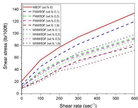
Figure 7. Shear stress vs shear rate of the WBDF, PNWBDF, and SNWBDF.
