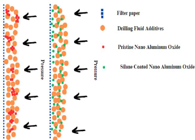
**Figure 14.** Dispersion and agglomeration of P-Al<sub>2</sub>O<sub>3</sub> and S-Al<sub>2</sub>O<sub>3</sub> NPs at the mud cake.
