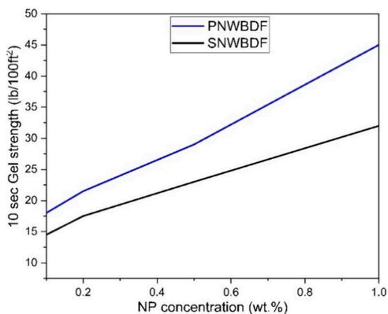
**Figure 11.** 10<sub>sec</sub> gel strength at different concentrations of P-Al<sub>2</sub>O<sub>3</sub> and S-Al<sub>2</sub>O<sub>3</sub> NPs.
