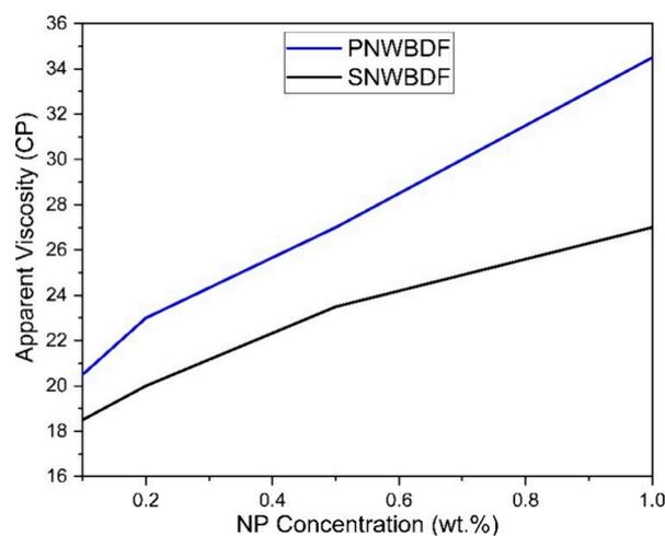
**Figure 9.** Apparent viscosity at different concentrations of P-Al<sub>2</sub>O<sub>3</sub> and S-Al<sub>2</sub>O<sub>3</sub> NPs.
