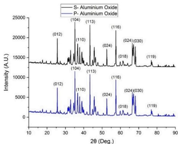
Figure 3. XRD analysis of P- $\text{Al}_2\text{O}_3$  and S- $\text{Al}_2\text{O}_3$  NPs.
